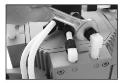
→ Use an open-ended wrench (w/f) 17 to remove the union nuts of the hose connections at the pump heads.
